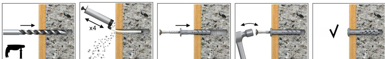
1. Drill a hole of required diameter.
