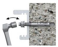
Lightly tap the throughbolt through the fixture into hole with a hammer, until fixing depth is reached
