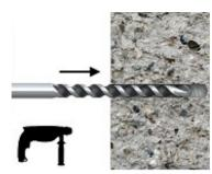
Drill a hole of required diameter and depth
