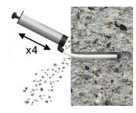
Clear the hole of drilling dust and debris (using blowpump or equivalent method)
