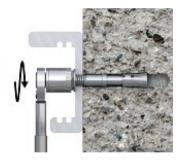
Tighten to the recommended torque
