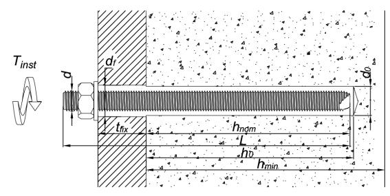
Table B1: Installation parameters – threaded anchor rod
