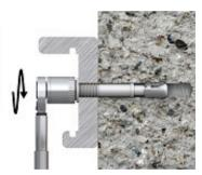
Tighten to the recommended torque
