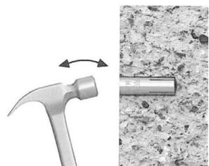
Insert the anchor (slotted end first).
