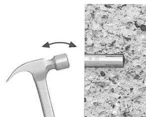
Insert the anchor (slotted end first).
