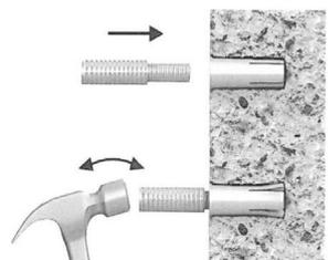
Use the setting tool to drive the internal wedge into the anchor.
